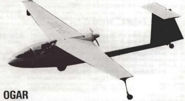
Two-seater Training Motor Glider Limbach Pusher engine 68 HP Glide angle 1:27 supplied with full set of instruments. British certification now complete. Demonstrator at Booker NOW
