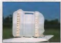
Figure 4. The measuring reservoir on top of the tailplane of the LS6. A slightly different and more practical method of marking the inverted scale, seen here on the right of the container, is described in the text. Also note the grip liner, just visible at the lower left corner of the bottle.
