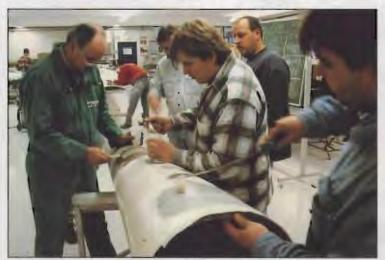
Learning how to repair holes in a tail cone made of fibre-glass.
