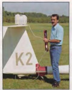
Figure 3. Cal Gillet (see acknowledgements) controlling the water flow of the measuring reservoir by means of the in-line drain cock of the small hose. The end of the hose is inserted into the tail ballast port.
