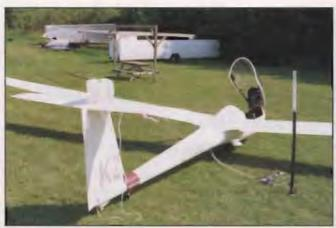
Figure 1b. The tail ballasting equipment shown in the drawing of Figure 1. Note that the standing pipe was placed closer to the glider than is advised in the text in order to 'concentrate' the various components of the system for illustrative purposes. Also note that the standing pipe is positioned downwind of the aircraft (as indicated by the red flag attached to the total energy probe) to prevent any water overflowing the top of the standing pipe to splatter the glider.
